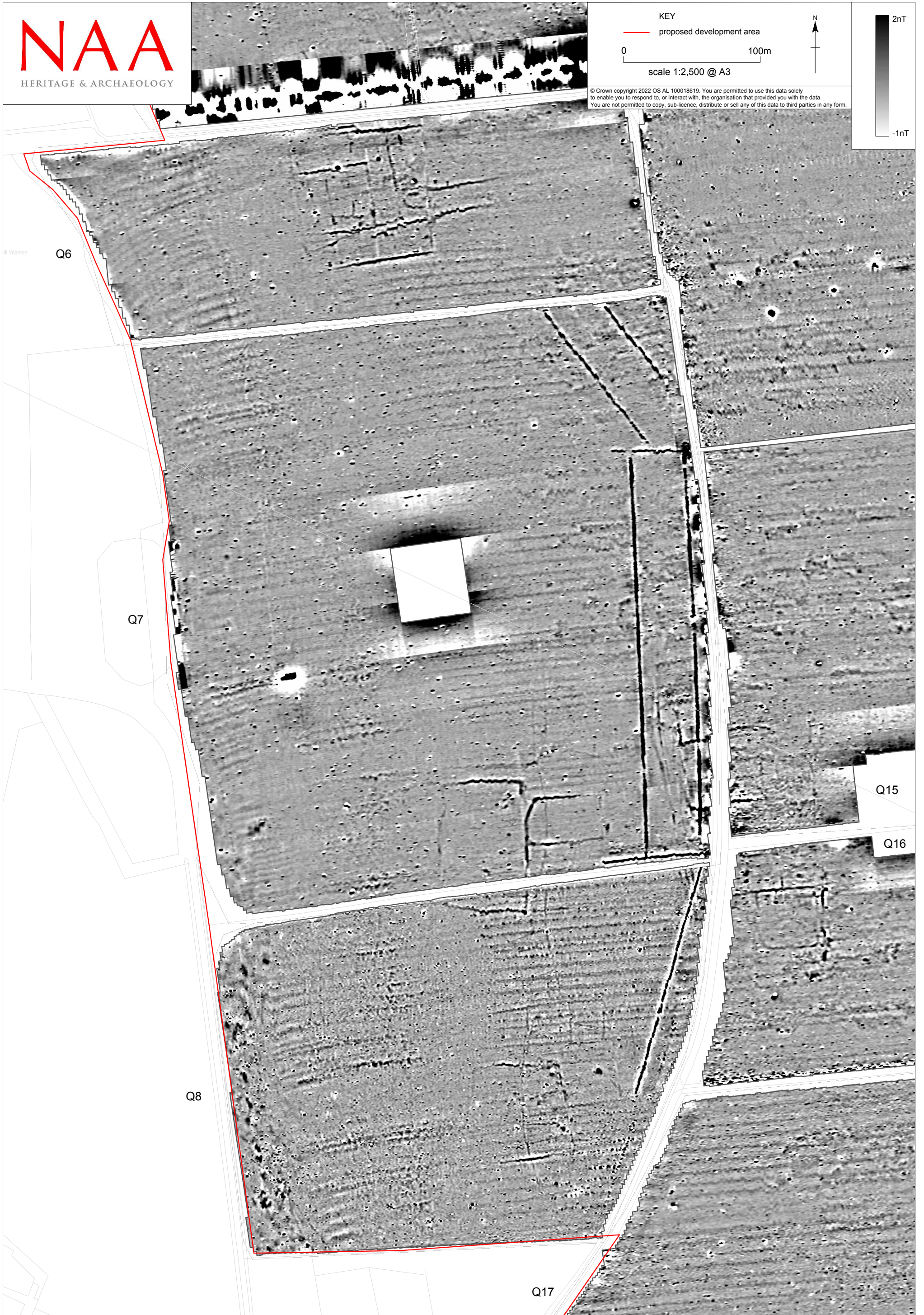
©NAA 2022 West Burton 3, West Burton Solar Scheme, Lincolnshire: processed greyscale plots of gradiometer survey results - Areas P7 and P8 Figure 16
